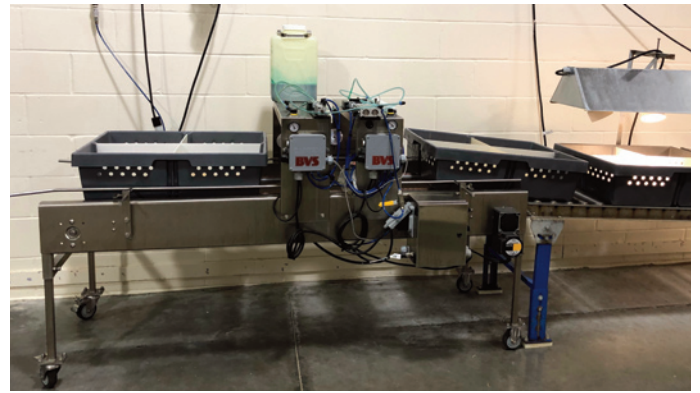
Figure 68. Spray and gel bar application with lights to promote preening post application
