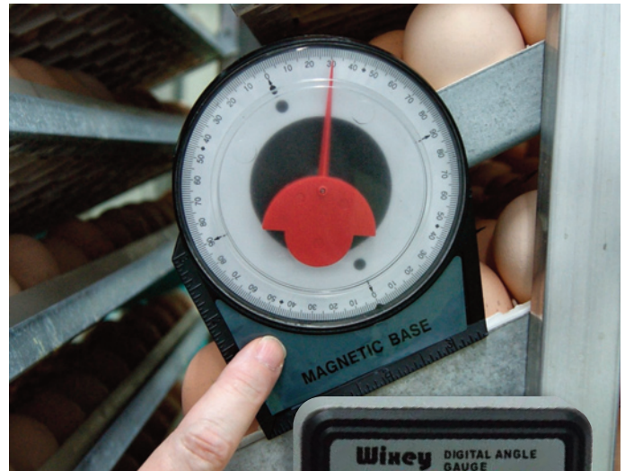
Figure 21a. Angle meter Figure 21b. Digital angle gauge. In both pictures the turning angle is too low, at around 30 degrees
