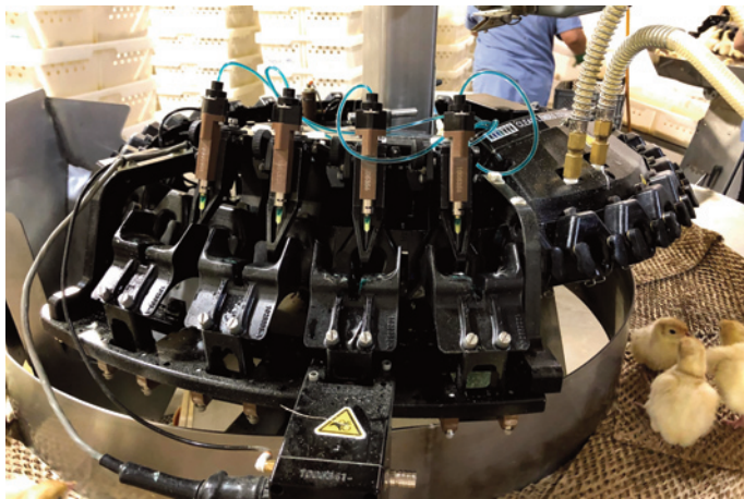
Figure 66. Fully automated injection with beak treatment
