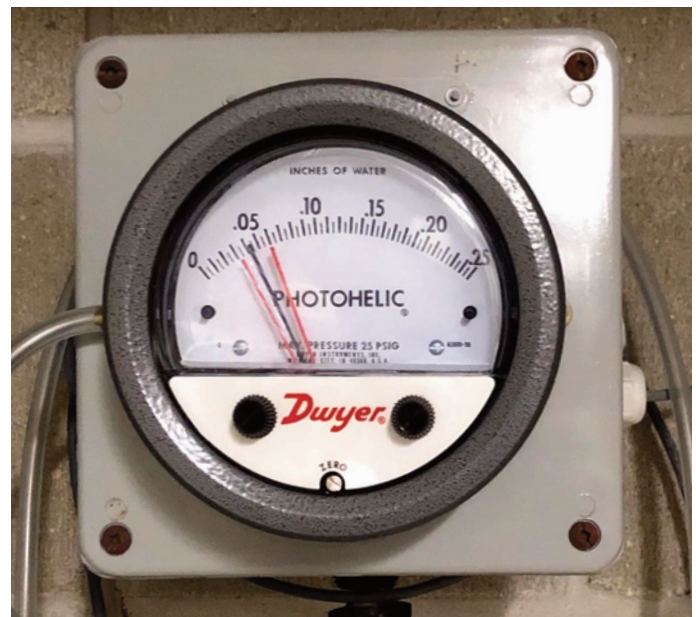
Figure 74. Dial meters can measure both positive and negative pressure
