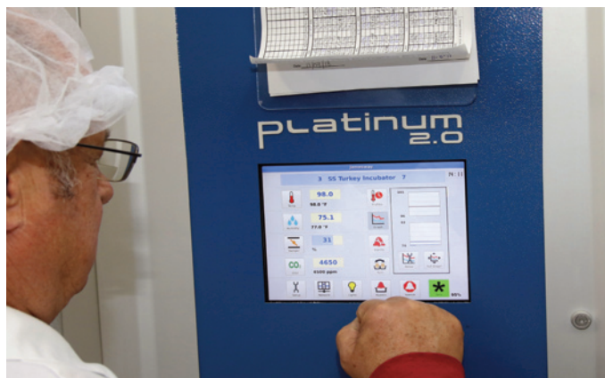
Figure 6. Pre-warming profiles programmed into an incubator
