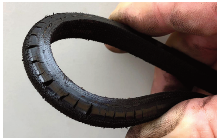
Figure 77. Worn fan belt
